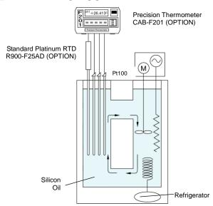
When comparison calibration of glass thermometer, then Pt 100 in above is changed to glass thermometer. Also wire connection from glass thermometer to CAB-F201 is removed.
